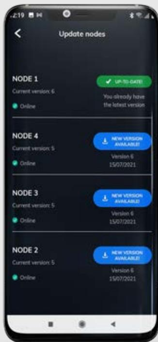
When process ends node will show a green circle and then a tick, as signal of successful update. On your device reload by swiping your finger from top to bottom of the screen, and you will see updated version on green on device screen.
