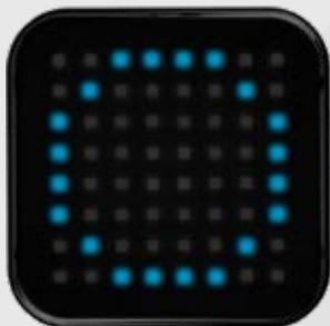
To reset nodes to factory settings you have to press node start button for 10 seconds and wait until blue circle appears.
